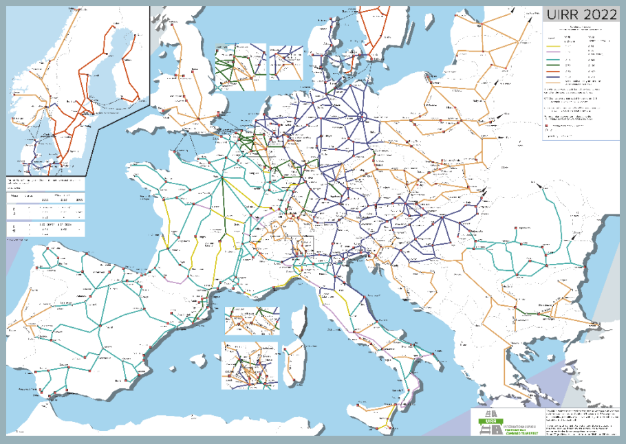
Figure 4: CT map of the codified lines for swap bodies and containers. All lines not colored yellow or light purple are suitable for transport of HC containers. A map in high resolution can be retrieved from [97].
