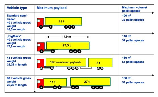
In the modelling process these LHV configurations were compared to the reference vehicle i.e. standard 40/44t/18m semi-trailer combination offering 33 pallet spaces and a payload of 26 tonnes.
